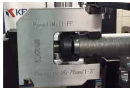
Inconel cladding removal application on 1" length
