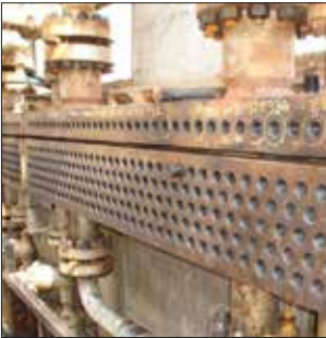
FinFan cooler before a maintenance
