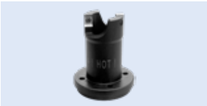
TFMH Tube facing milling head for tubes made of any type of material. Utilizes 6% cobalt inserts. → TABLE PAGE 58
