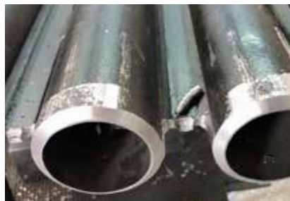
Membrane removal application on 1" length
