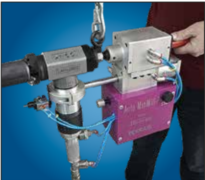
SPEED ADJUSTMENT VALVE SAV-500 The solution for all pneumatic drove beveling machines. Allows adjusting cutting speed to suit to the machined tube diameter.
