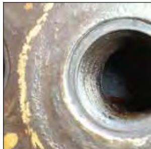
Plug hole before re-machining the gasket seat
