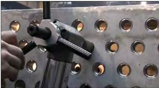
☞ Trimming tubes safely and efficiently. Machine locks securely both to the tube and the plug thread of the water box.
