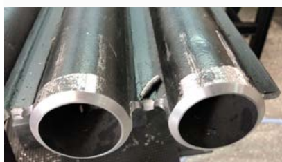
Membrane removal application on 1" length
