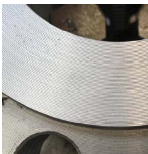
Single line gramophone groove (50 grooves per 1 inch)
