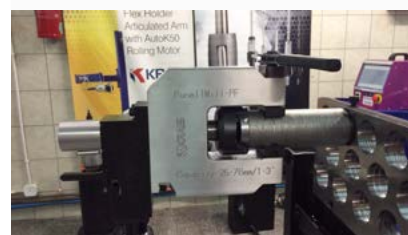
Inconel cladding removal application on 1" length
