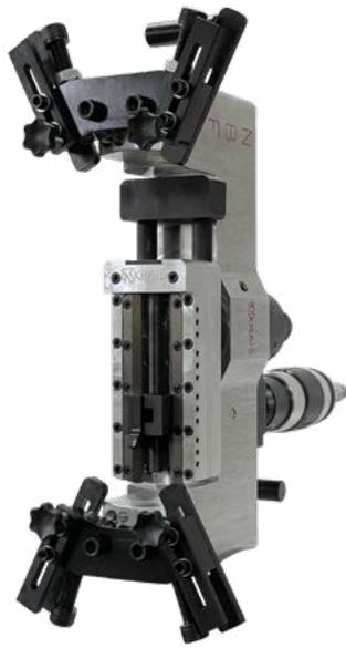
The standard locking system consists of two jaws. One of them is a stabilizing jaw with two adjustable screws to fit the outer diameter of the flange. The second jaw has three clamping screws. Both jaws are equipped with pair top pads for levelling on the sealing surface of the flange. Pads at the bottom, are for tension the machine to the flange surface. Pads help to fix the machine in any position and protect it from falling out of the flange in case of a collision.
