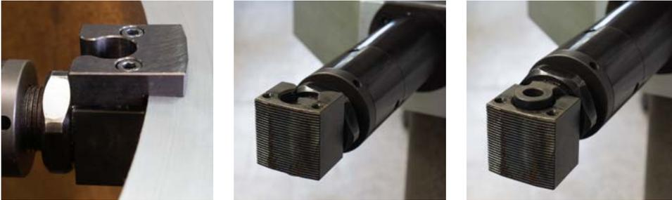
IMFM40 Special jaw set for easy and quick levelling and centering machine. A special mechanism allows convenient adjustment of the mounting plane relative to the pipe. Built-in self-centering locking system significantly facilitates the coarse setting of the machine.
