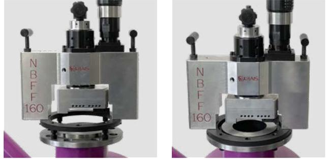
Additional, special flange type locking system is made to suit the application more. NBFF machine is still mounted on the flange outside diameter, but the locking system is equipped with additional studs to be mounted in the flange holes to provide easy operation and perfect centring.
