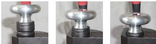
The Modul is equipped as standard with feed gearbox in order to generate both, fine or coarse surface finish by simple switch on the gear box.
